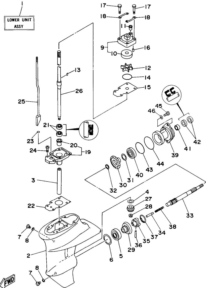
FIG. 14 LOWER CASING. DRIVE 1 IMPULSOR E INFERIOR 1
