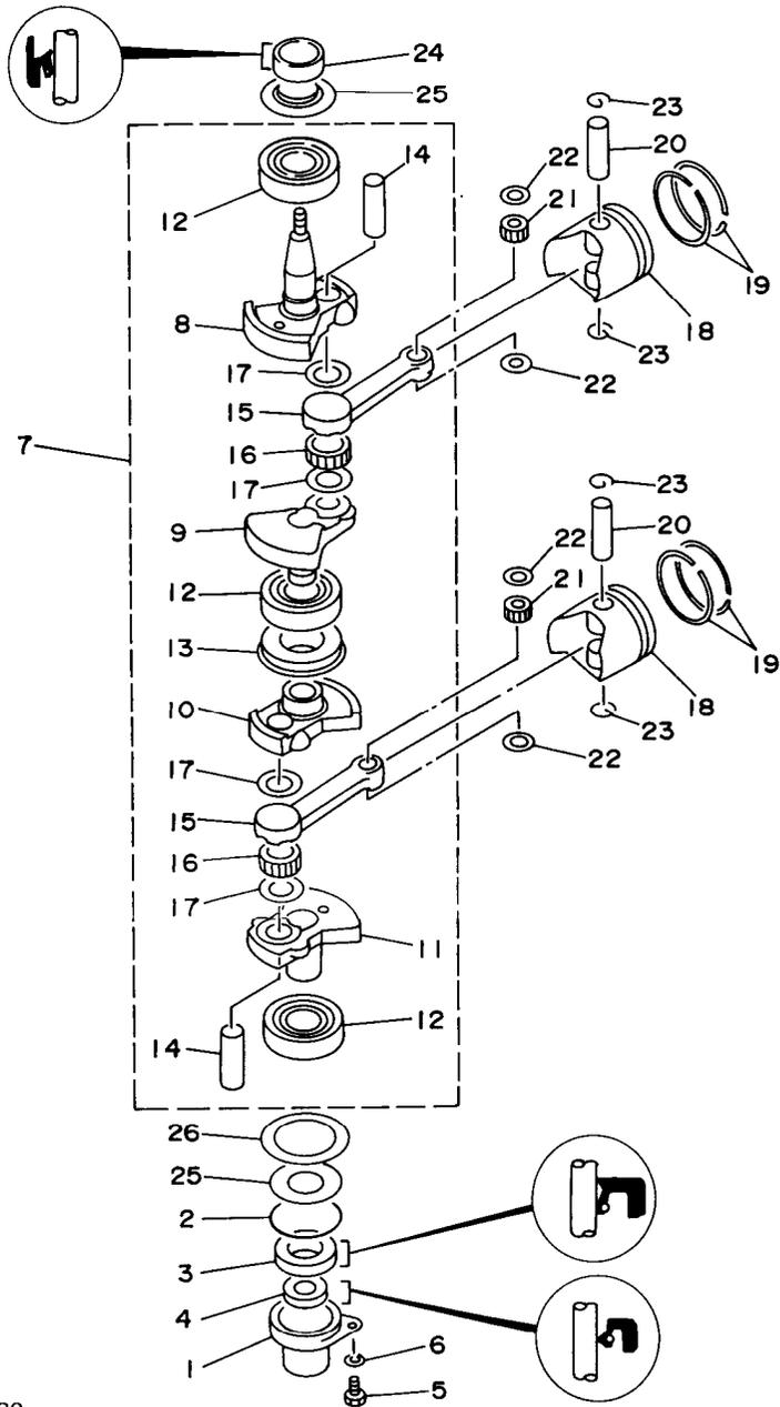
FIG. 2 CRANKSHAFT. PISTON
