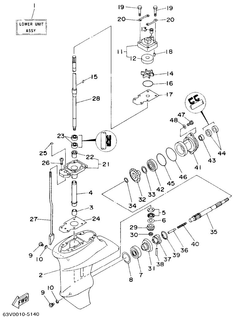
FIG. 19 LOWER CASING. DRIVE 1 IMPULSOR E INFERIOR 1
