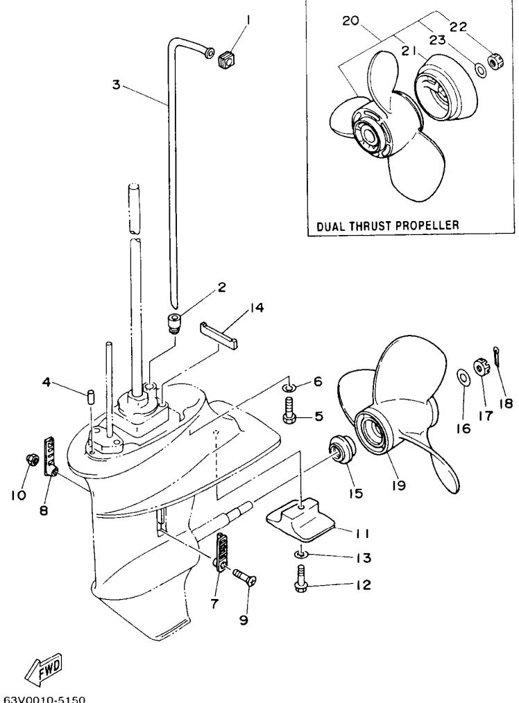
**FIG. 20 LOWER CASING. DRIVE 2 IMPULSOR E INFERIOR 2**
