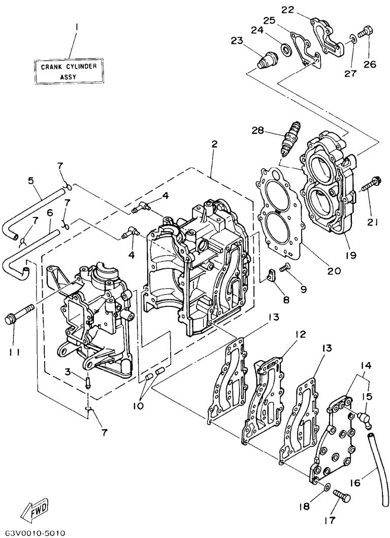
FIG. 1 CYLINDER. CRANKCASE CYLINDRO. CARTER
