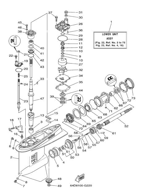
FIG. 22 LOWER CASING & DRIVE 1
