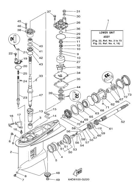
FIG. 22 LOWER CASING & DRIVE 1
