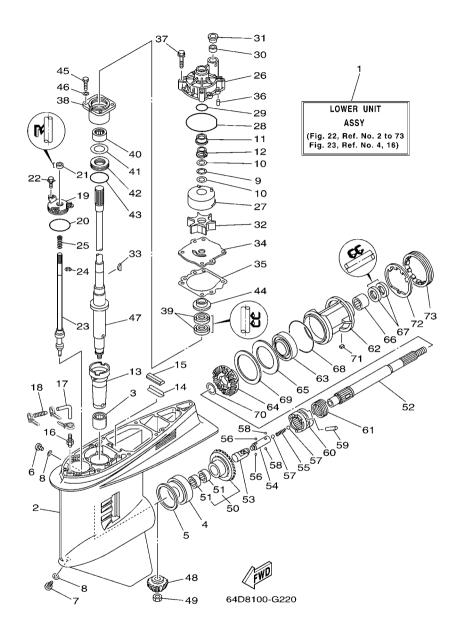
FIG. 22 LOWER CASING & DRIVE 1
