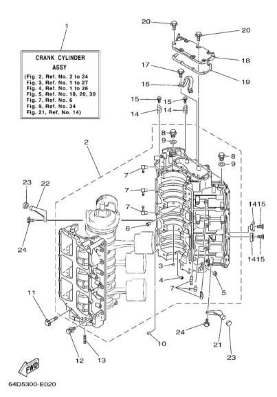
FIG. 2 CYLINDER & CRANKCASE 1
