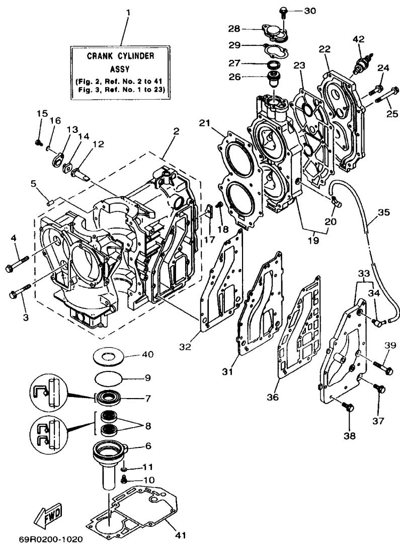
FIG. 2 CYLINDER. CRANKCASE
