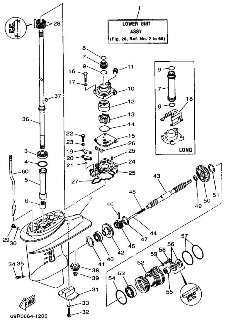
**FIG. 20 LOWER CASING. DRIVE 1**
