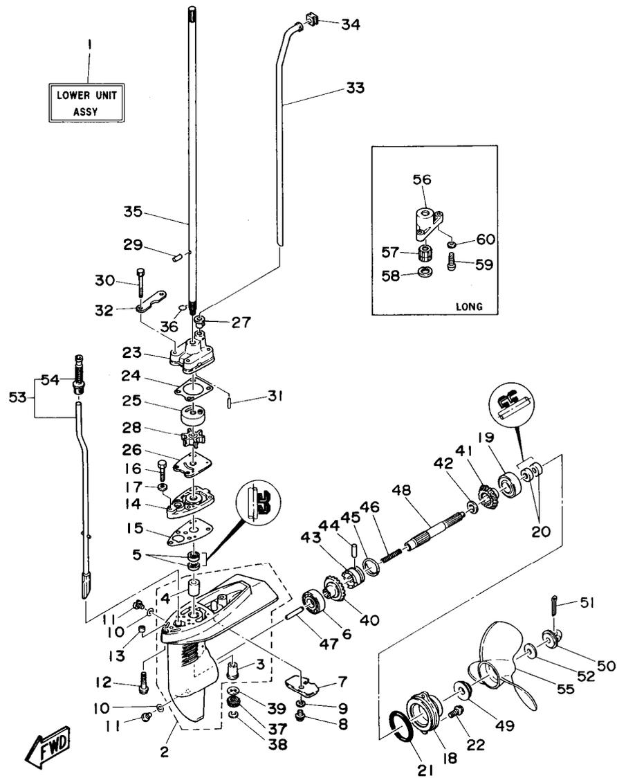
FIG. 8 LOWER CASING. DRIVE 1 IMPULSOR E INFERIOR 1
