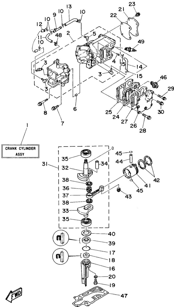
FIG. 1 CYLINDER. CRANKCASE CYLINDRO. CARTER
