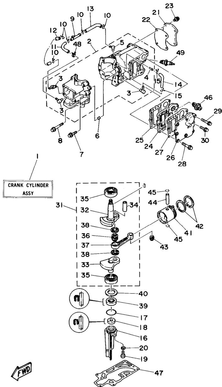
FIG. 1 CYLINDER. CRANKCASE CYLINDRO. CARTER
