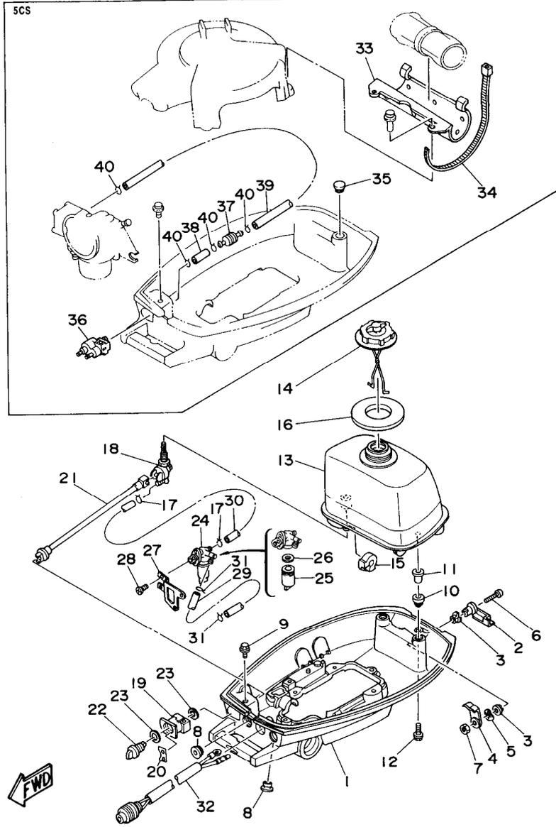
FIG. 5 BOTTOM COWLING CUBIERTA INFERIOR
