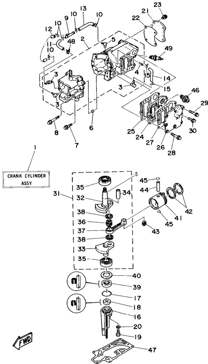
FIG. 1 CYLINDER. CRANKCASE CYLINDRO. CARTER
