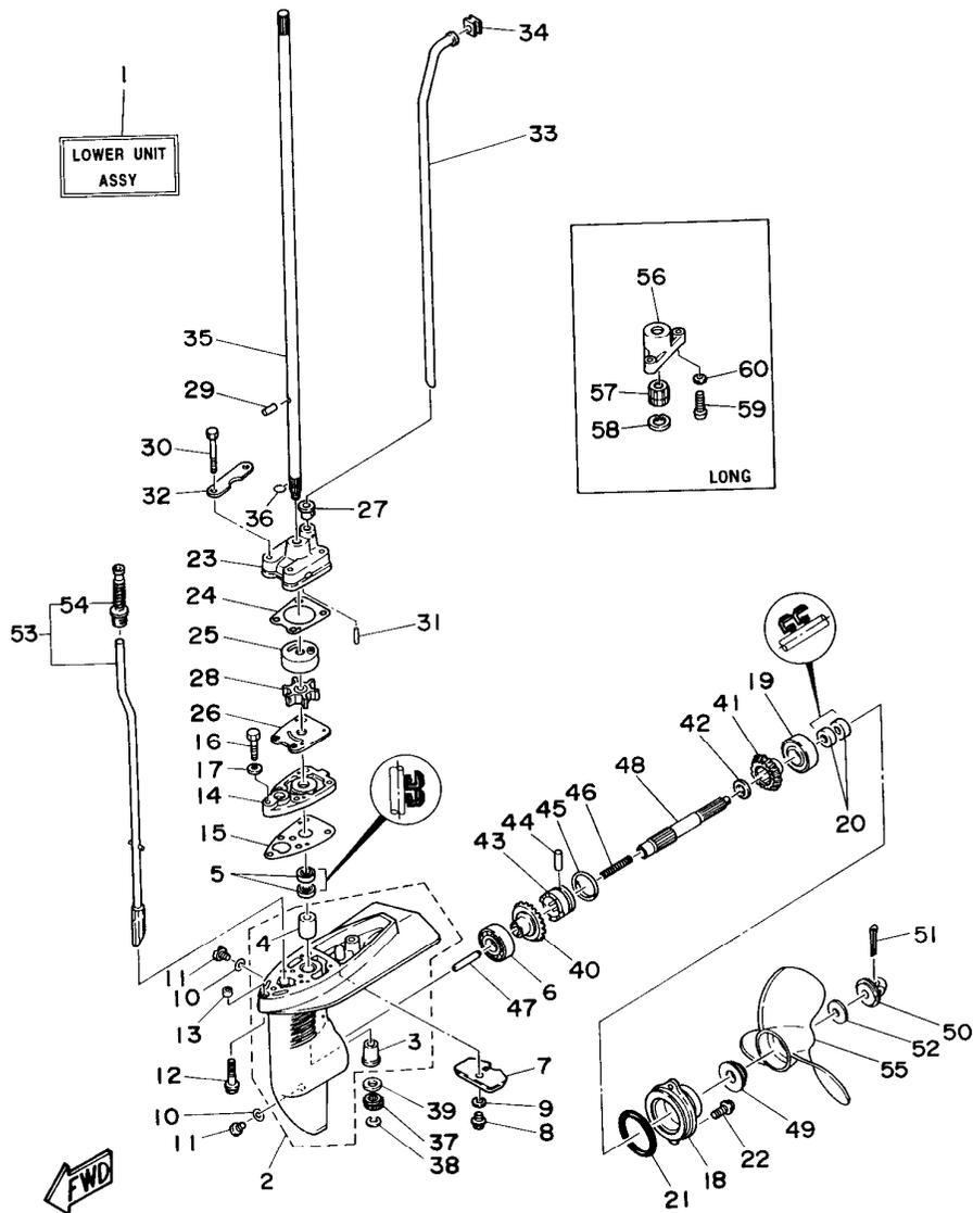
FIG. 8 LOWER CASING. DRIVE 1 IMPULSOR E INFERIOR 1
