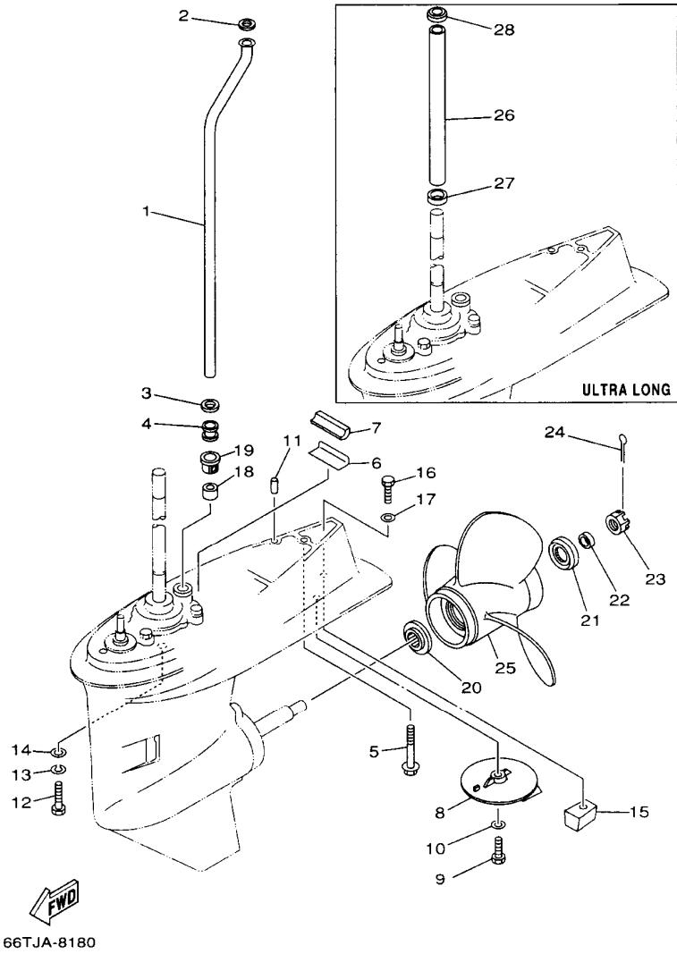
FIG. 24 LOWER CASING, DRIVE 2 IMPULSOR E INFERIOR 2
