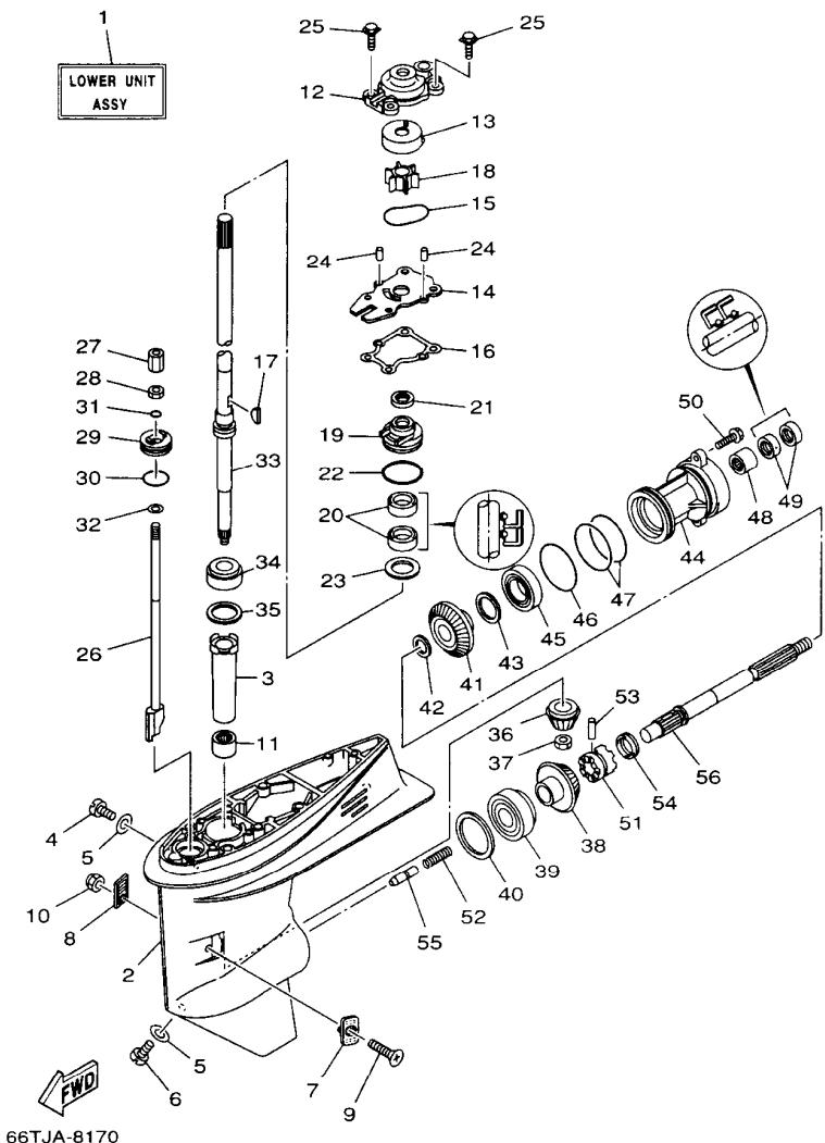
FIG. 23 LOWER CASING, DRIVE 1 IMPULSOR E INFERIOR 1
