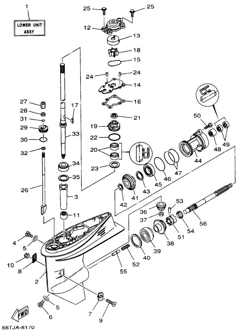
**FIG. 23 LOWER CASING, DRIVE 1      IMPULSOR E INFERIOR 1**
