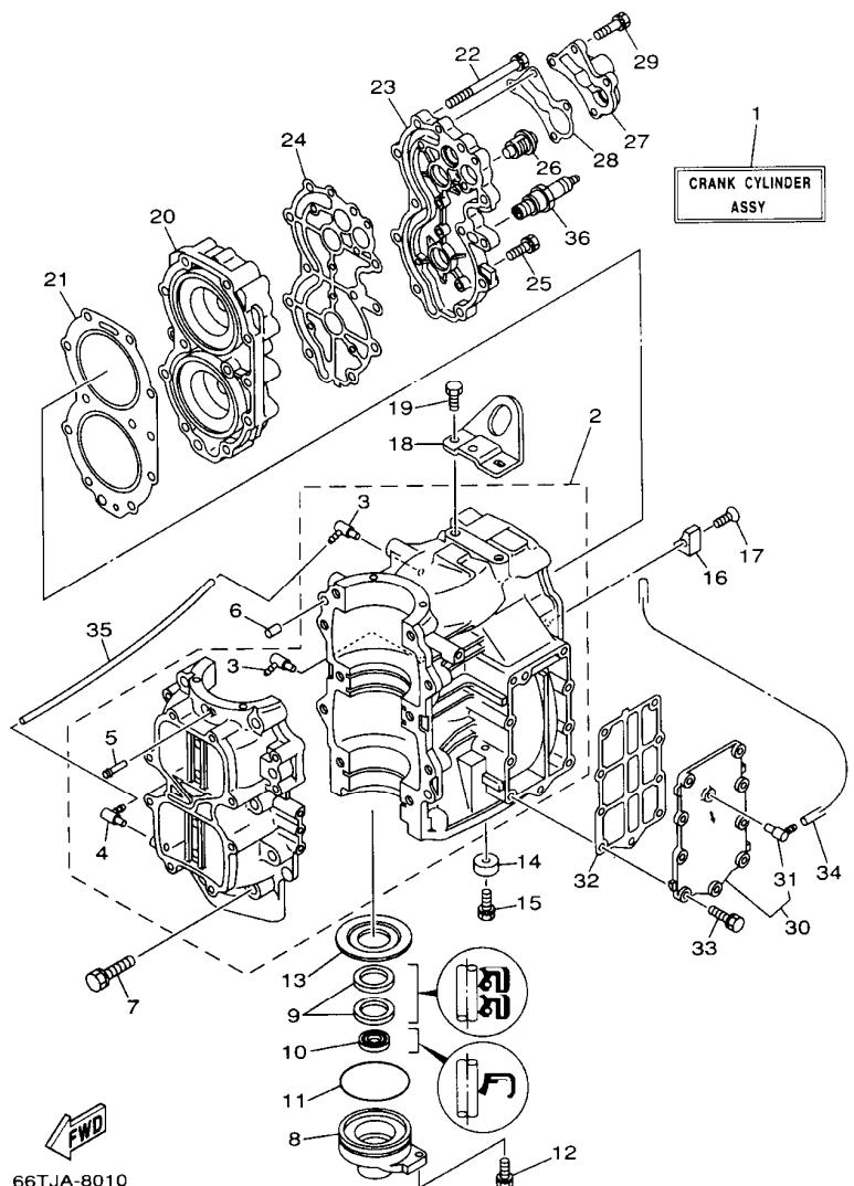
FIG. 1 CYLINDER. CRANKCASE CYLINDRO. CARTER
