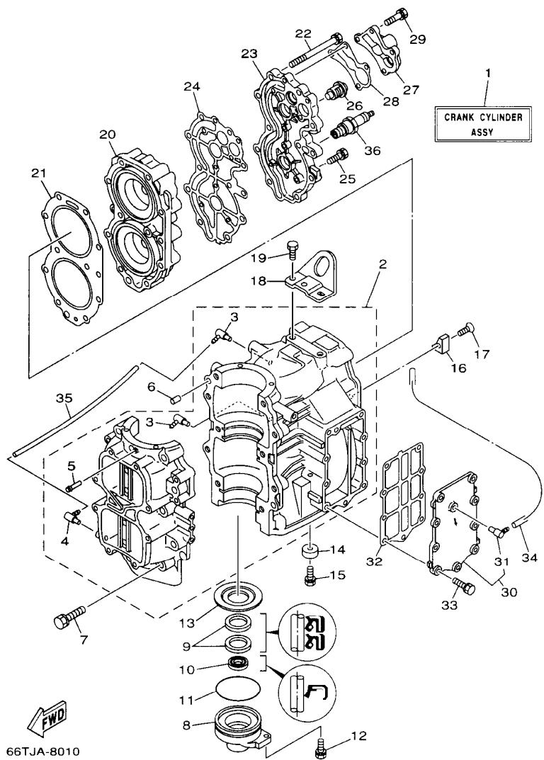
FIG. 1 CYLINDER, CRANKCASE
