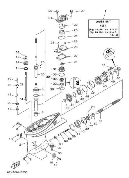
FIG. 25 LOWER CASING & DRIVE 1
