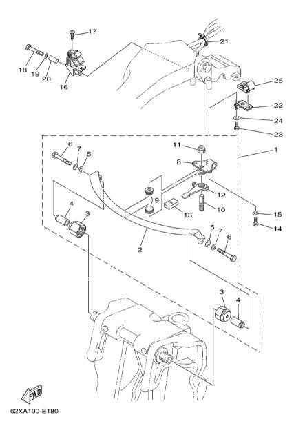
FIG. 18 STEERING FRICTION
