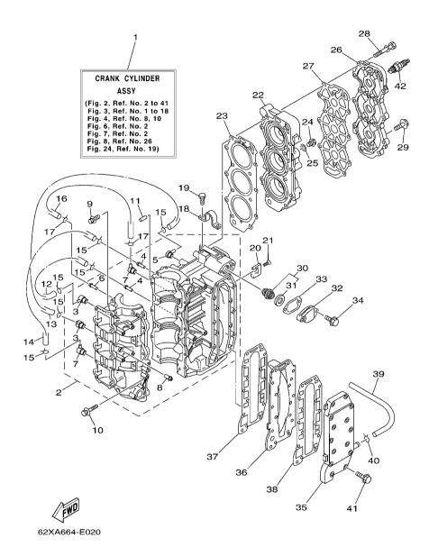
FIG. 2 CYLINDER & CRANKCASE
