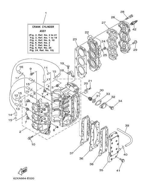
FIG. 2 CYLINDER & CRANKCASE
