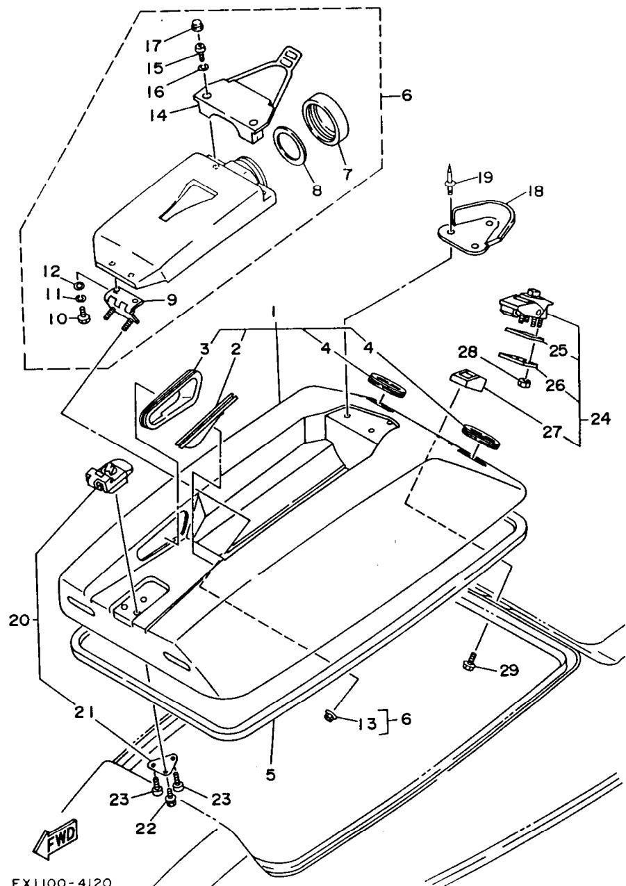
FIG. 12 ENGINE HATCH
