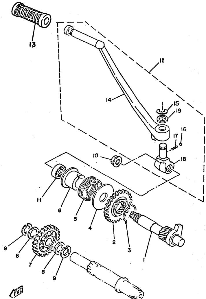
FIG. 09 – EIXO DO PEDAL DE PARTIDA
