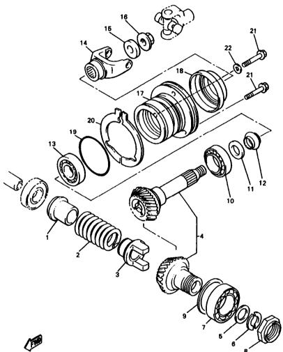
FIG. 17 MIDDLE DRIVE GEAR REF. PART NO. DESCRIPTION
