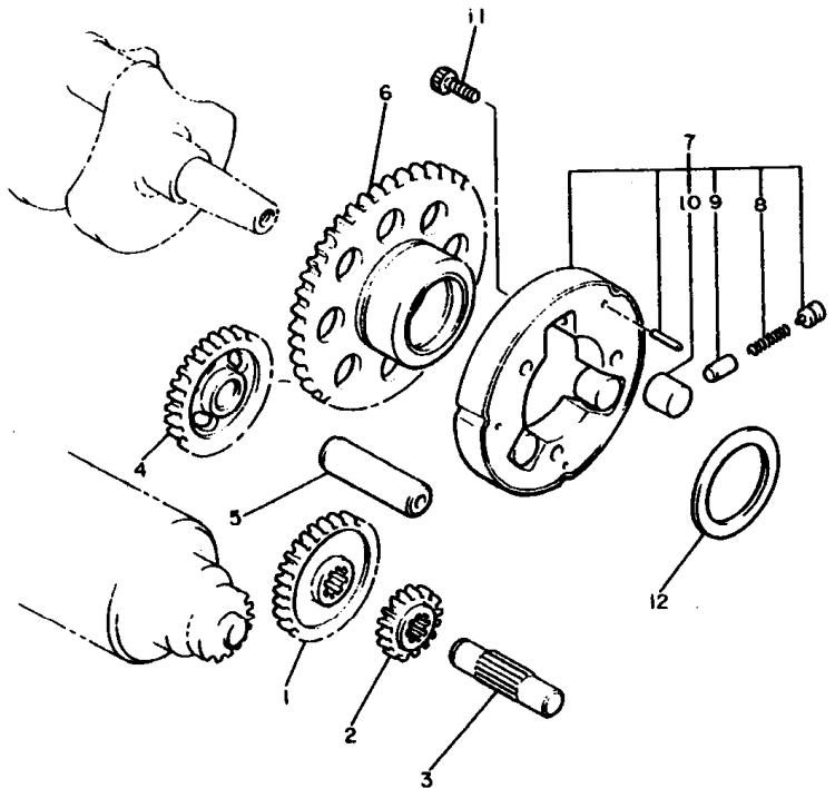
**FIG. 14 STARTER CLUTCH**
