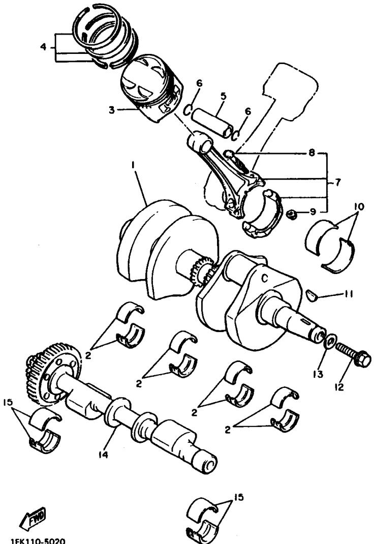
FIG. 2 CRANKSHAFT. PISTON
