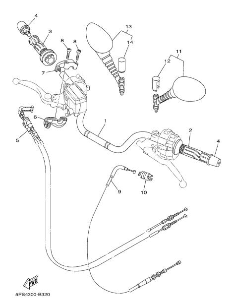
FIG. 32 STEERING HANDLE & CABLE
