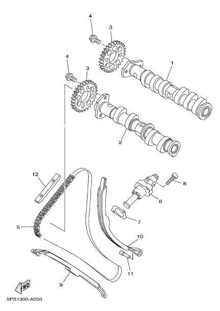
FIG. 5 CAMSHAFT & CHAIN
