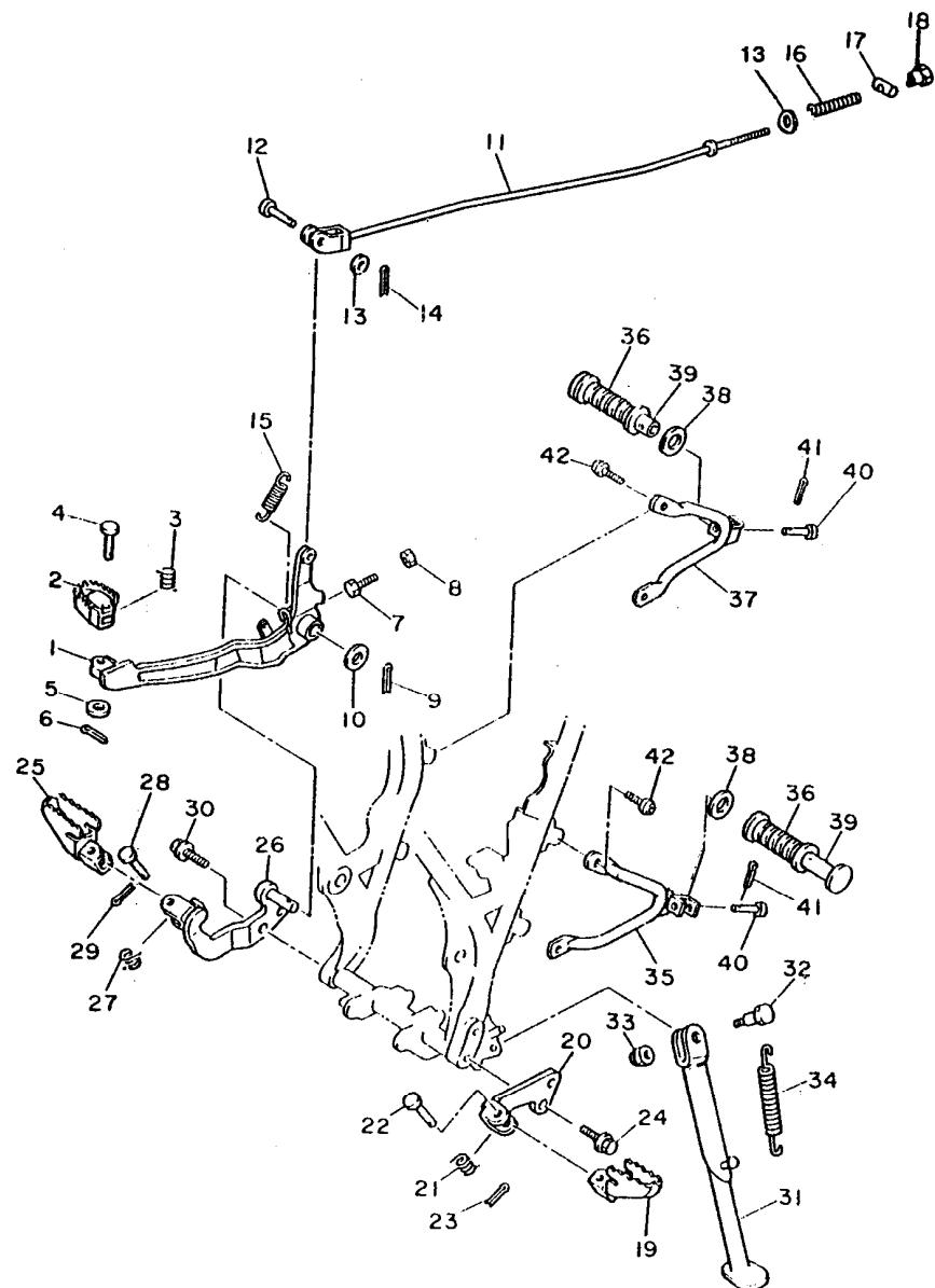
FIG. 30 – PEDAL DE FREIO, ESTRIBO E CAVALETE LATERAL
