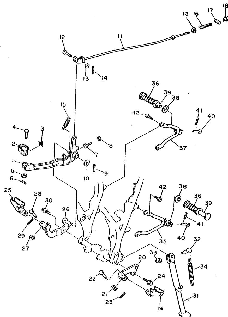
FIG. 30 – PEDAL FREIO, ESTRIBO E CAVALETE LATERAL
