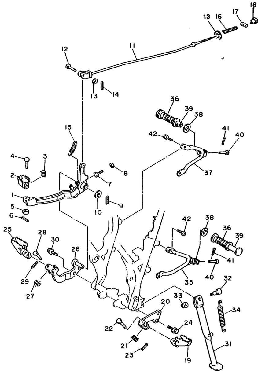
FIG. 30 - PEDAL DE FREIO, ESTRIBO E CAVALETE LATERAL
