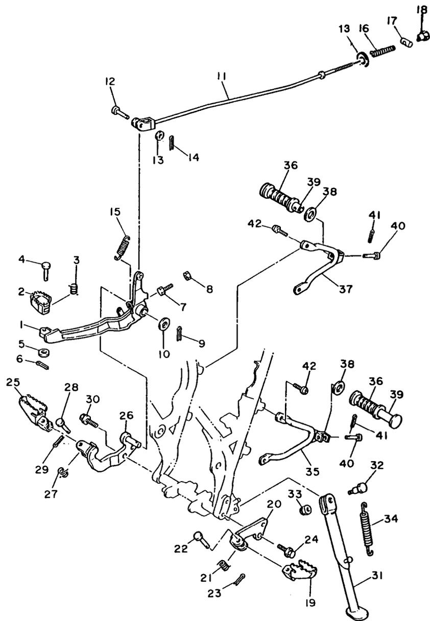
FIG. 30 - PEDAL FREIO, ESTRIBO E CAVALETE LATERAL (Cont.)
