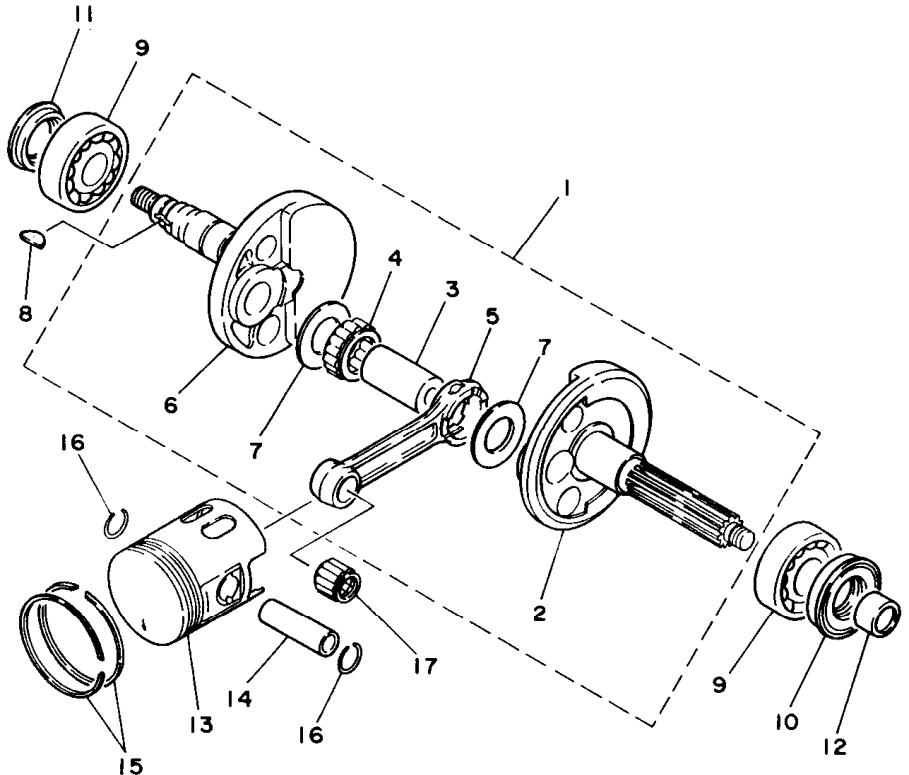
FIG. 2 CIGUENAL. PISTON CRANKSHAFT. PISTON
