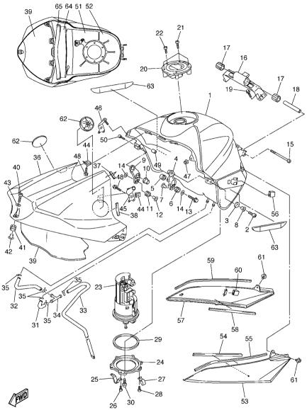
FIG. 28 FUEL TANK 5VY7 PART NO. DESCRIPTION REMARKS 26 98907-05008 SCREW, BIND 2 CLAMP 27 90461-10010 1 SCREW, BINDING 28 90154-05012 1 29 5JW-24486-00 O-RING 1 30 90110-05014 BOLT, HEXAGON SOCKET HEAD 6 31 5VY-24315-00 PIPE 5 1 32 5VY-24316-00 PIPE 6 1 33 5VY-24317-00 PIPE 7 1 34 90413-07007 WAY 3 1 35 90467-09006 CLIP 5
