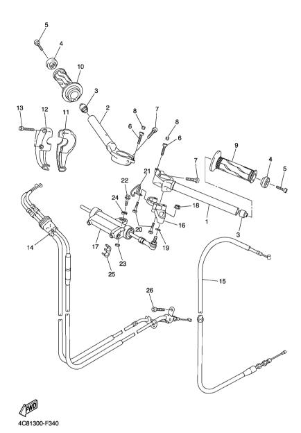
FIG. 34 STEERING HANDLE & CABLE
