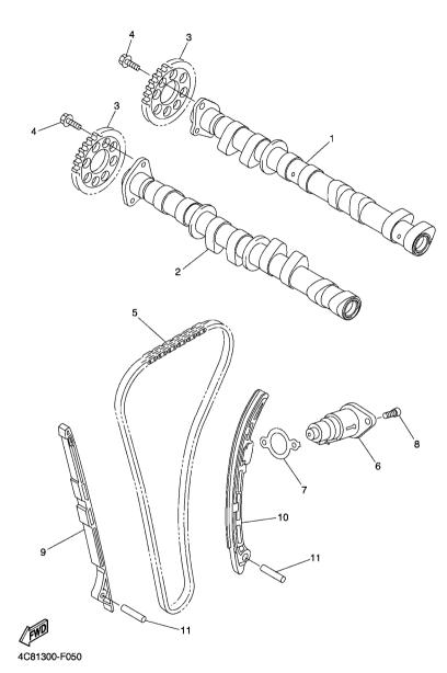
FIG. 5 CAMSHAFT & CHAIN
