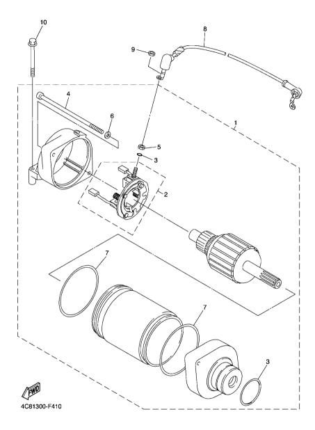
FIG. 41 STARTING MOTOR
