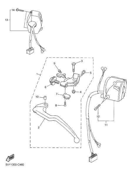
FIG. 46 HANDLE SWITCH & LEVER
